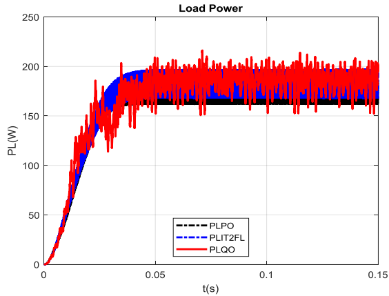
Fig 11. Comparative analysis of Load power using P&O, IT2FL, and QO-based MPPT controllers
