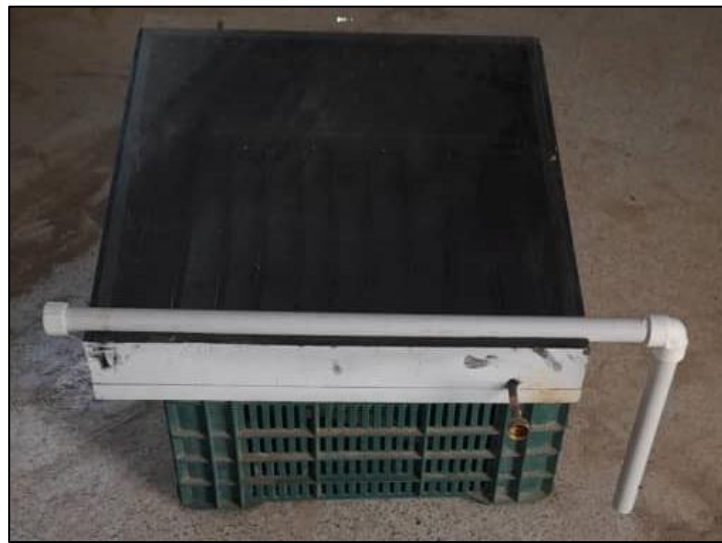
Fig 2. Fully assembled single-slope solar still with integrated water collection system.
